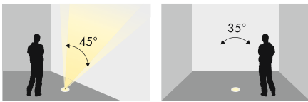
Asymmetrische Linse 45°/35° / Asymmetrical lens 45°/35°
